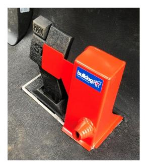
2. With the lock removed place the cover over the accelerator pedal.
