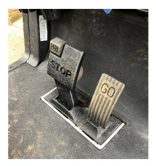
1. Ensure the brake is applied to the buggy.
