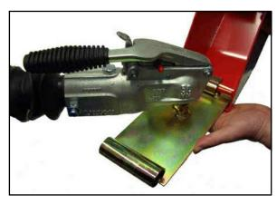
2a. Locate Dummy Ring. Open the hitchlock and offer up the bottom plate at an angle to the coupling. Please Note: The red lever on the hitch head must not be engaged, i.e. the hitch handle must be down.
