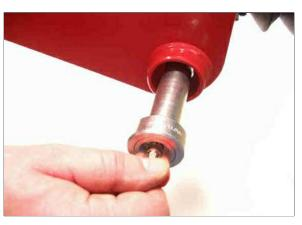
**4. Locking.** The lock bolt is inserted and pushed fully into its hardened steel cup which is permanently retained by the plastic holder on the side. Turn key 1/4 turn clockwise to lock and remove key. Push on plastic cap to protect lock.
