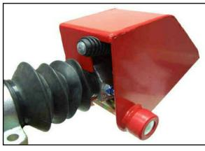
**3. Lower The Hood.** Rotate the top cover to enclose the hitch head.
