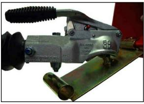
**2b** Twist the bottom plate until it is in line with the hitch head avoiding the fixing as the hitchlock is rotated.
