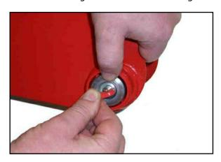
1. To Remove Lock Bolt. Hold head of bolt with thumb to prevent turning. Insert the key and turn ¼ turn anti-clockwise. Pull out lock bolt with key. Place aside carefully. Do not allow dirt to enter lock.
