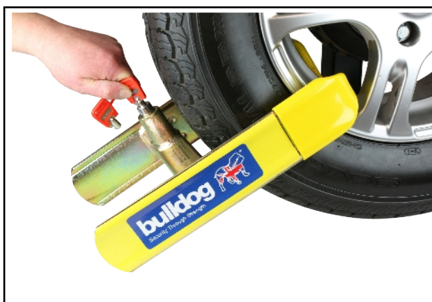
4. To remove clamp, insert key, rotate 1/2 turn, pull on key and/or press inner and outer arms together until lock pops out.
