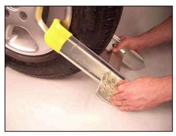
**2.** Slide inner and outer arms together, ensuring pointed outer arm fits into recess or hole in wheel. Position padlock above the hole closest to the outer arm and turn the key to lock.
