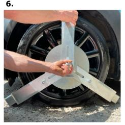
Fully extend the arms of the clamp and position the assembly around the base of the wheel. Push the clamp back and then lift the central nut and disc assembly to the centre of the wheel. Whilst still holding the central nut move the top arm into a vertical position.
