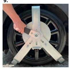
Once the top arm is in position keep hold of the central nut and pull the right hand arm tight into the tyre, followed by the left hand arm. Tighten the central nut by hand to hold the disc and arm in position then fully tighten using the spanner (6).
